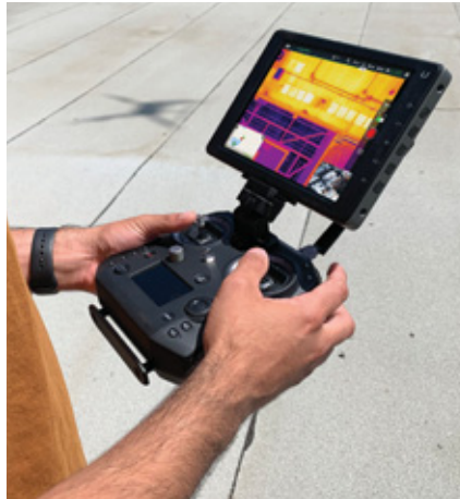
Using drones equipped with thermal sensors allows customers to proactively find moisture under a roof membrane and potential areas of energy loss. PHOTO COURTESY OF ZEITVIEW.
