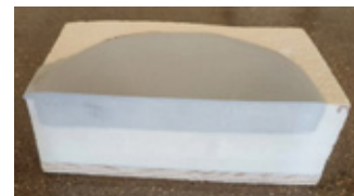
A lab prototype that mimics a ponded area on a roof. Scientists filled in the area with ECO-LEVEL compound to test its properties.
