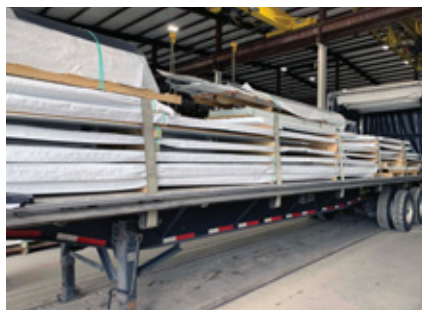
Exposed fastener panels loaded on a flatbed trailer. Panels nest for more cost-efficient shipping. PHOTOS COURTESY OF MCELROY METAL.
