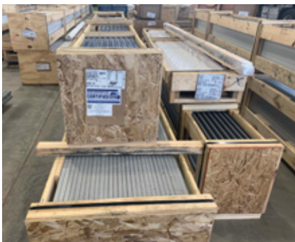
Concealed fastener panels require the construction of solid wooden crates. Packaging is more extensive than through-fastened panels, resulting in higher shipping costs.
