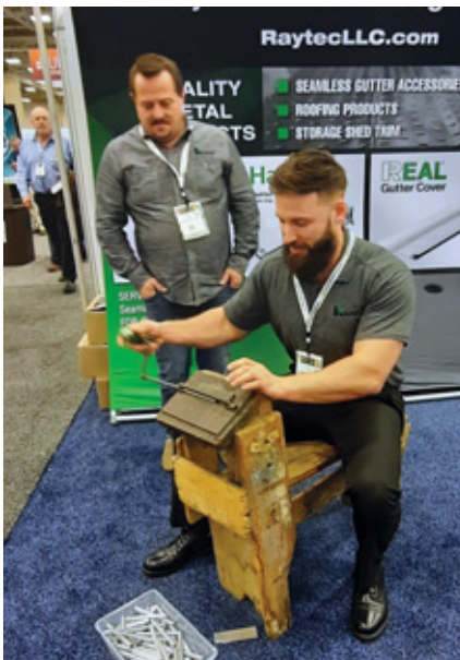
Raytec Manufacturing exhibited an antique bench used for making ferrules. Tag Saunders looks on as Jordan Fox operates the machine.
