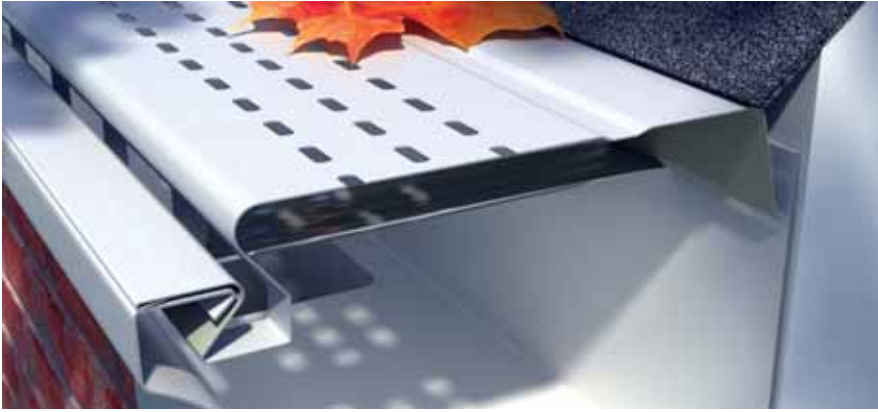
The E-Z-HydroClean High Capacity gutter guard from Midwest Enterprises. The holes admit some of the water into the gutter, slowing the flow, while the rest flows around the nose into the gutter.
