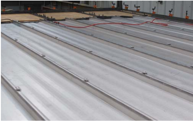
A demonstration of ASTM E1592, used to determine maximum/ultimate wind load, which in turn is used to specify the appropriate design wind load. Photos courtesy of S-5!
