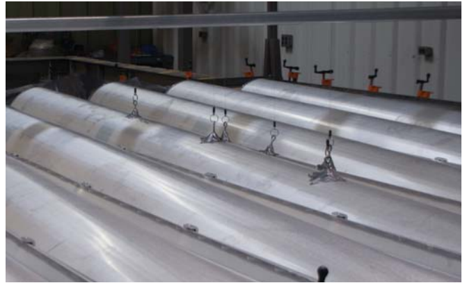
A demonstration of ASTM E1592, used to determine maximum/ultimate wind load, which in turn is used to specify the appropriate design wind load. Photos courtesy of S-5!
